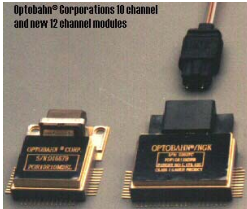
10 and 12 Channel, 2.5 Gbit/sec/fiber transceivers Optobahn
