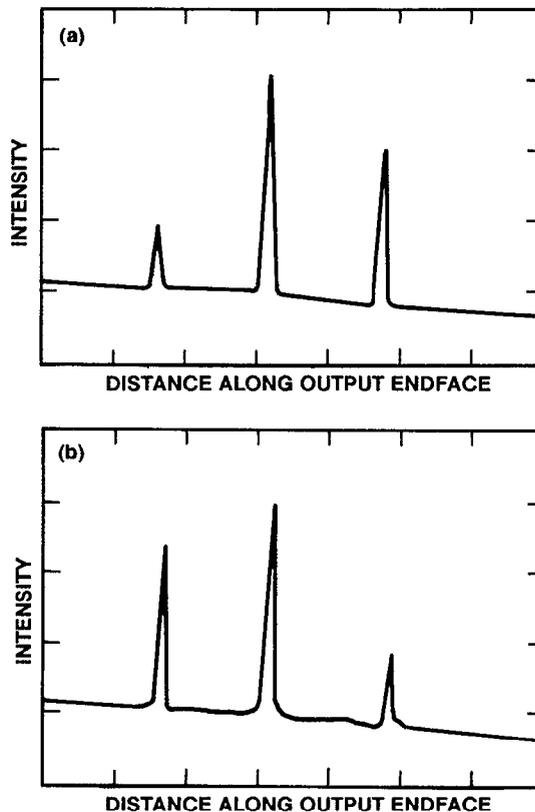
FIG. 3. Complementary switching between taps (arbitrary units). (a) With voltage applied to the left channel, light is switched into the right channel. (b) With voltage applied to the right channel, light is switched into the left channel.
