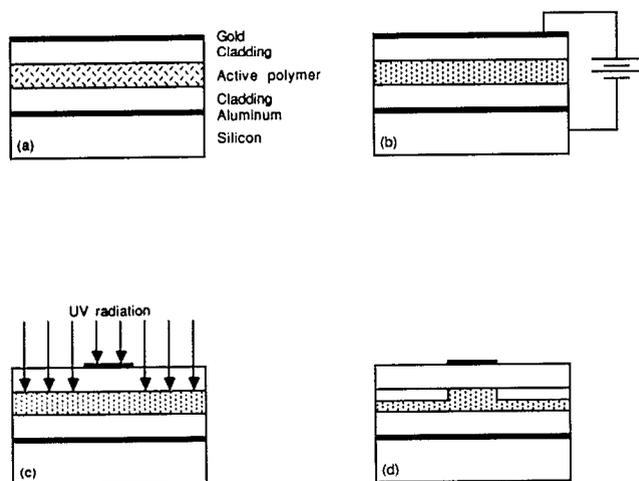
FIG. 2. Device structure and processing steps. (a) Device structure after deposition of waveguiding and metal layers, (b) active molecule alignment by poling, (c) selective photobleaching with a gold mask, (d) final electro-optic channel waveguide.
