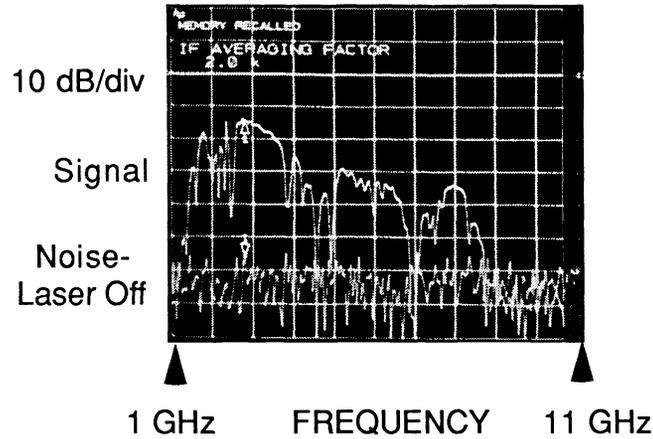
Figure 9. Optical Modulation Response of Mach-Zehnder #152 From 1 to 11 GHz
