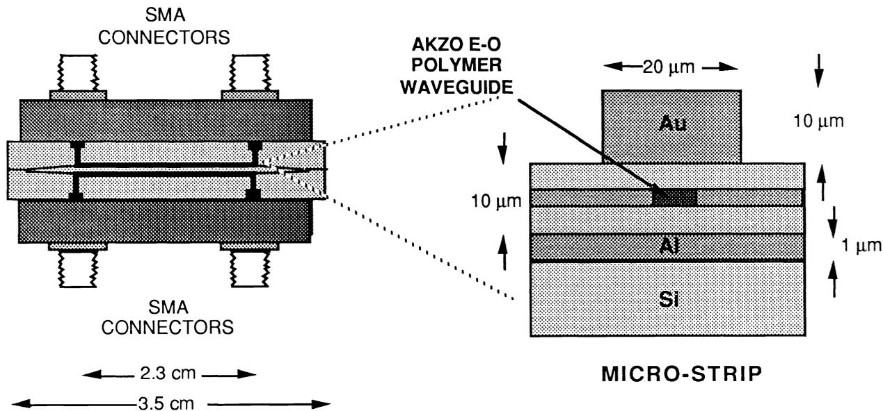
Figure 7. Schematic Diagram of Mach-Zehnder Modulator #152
