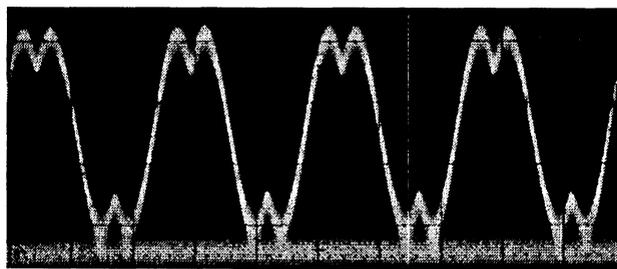
Figure 8. Modulation Depth Measurement of Mach Zehnder 152
