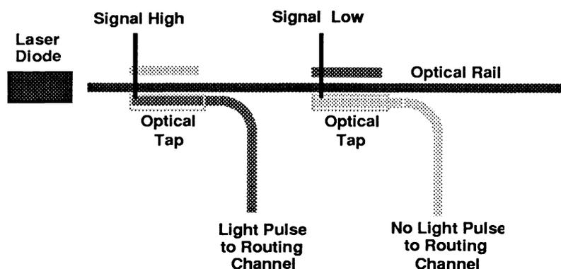
Figure 2. Schematic View of a Railtap for Optical Interconnects.
