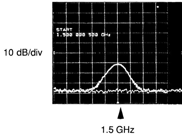
Figure 11. Heterodyne Signal at 1.5 GHz From Drive Signals at 18.5 and 20 GHz
