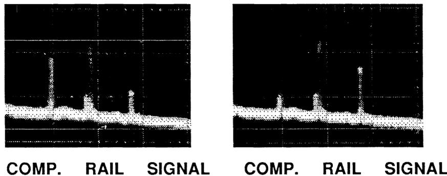
Figure 4. Intensity Line Scan Of the Railtap Endface Showing Complementary Modulation.
