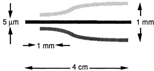
Figure 3. Dimensions of a Sample Single Element Railtap.
