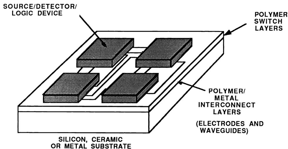
Figure 1. Schematic Diagram of an Optical Multi-Chip Module Based on Electro-Optic Polymers.
