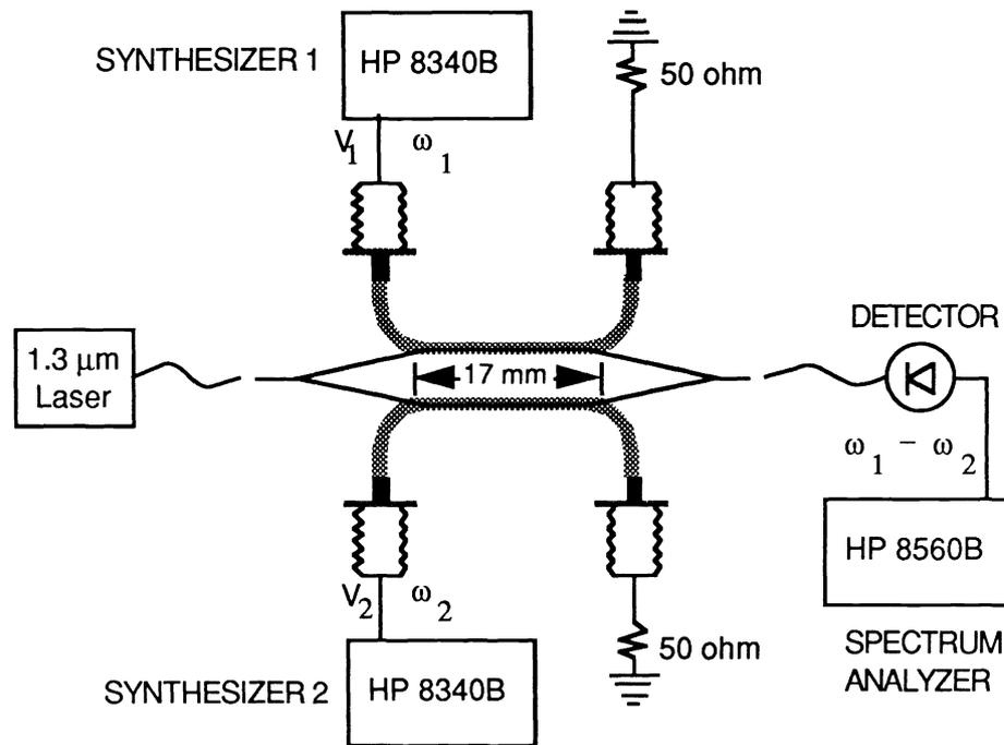
Figure 10. Heterodyne Measurement of the High Frequency Response of Device #152
