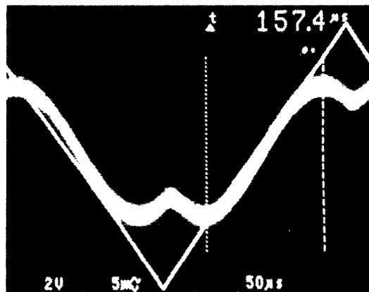
FIG. 3. Response of EO polymer-based Mach-Zehnder modulator to triangular waveform, demonstrating a half-wave voltage of  $V_\pi = 9$  V.
