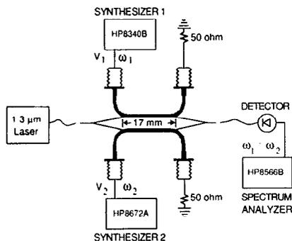
FIG. 2. Schematic showing dual-electrode measurement technique for Mach-Zehnder modulator fabricated with an EO polymer. Synthesizers 1 and 2, at different frequencies ( $\omega_1$  and  $\omega_2$ ), produce an optical signal at the difference frequency ( $\omega_1 - \omega_2$ ) which is observed on the spectrum analyzer.
