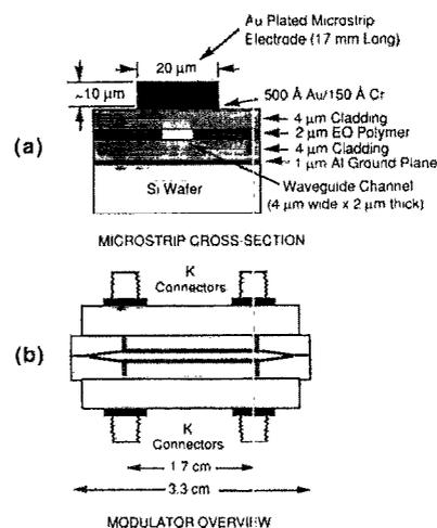
FIG. 1. (a) Cross section of the photobleached EO polymer optical waveguide and microstrip drive electrode from one arm of the Mach-Zehnder device, and (b) overview of the high-speed Y-branch Mach-Zehnder integrated optic modulator.
