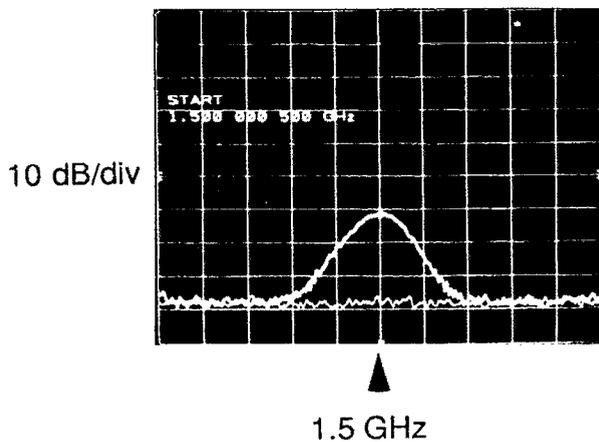
FIG. 4. Optical output signal at 1.5 GHz from electrode drive signals at 18.5 and 20 GHz, demonstrating device modulation at 20 GHz.
